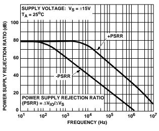
FIGURE 36. POWER SUPPLY REJECTION RATIO vs FREQUENCY
