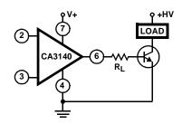
FIGURE 4. METHODS OF UTILIZING THE V<sub>CE(SAT)</sub> SINKING CURRENT CAPABILITY OF THE CA3140 SERIES
