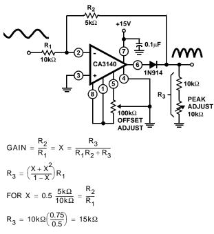
$20V_{P-P}$  Input BW (-3dB) = 290kHz, DC Output (Avg) = 3.2V
