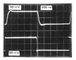
Top Trace: Output; 50mV/Div., 200ns/Div. Bottom Trace: Input; 50mV/Div., 200ns/Div. FIGURE 28B. SMALL SIGNAL RESPONSE
