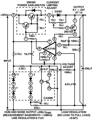
FIGURE 16. REGULATED POWER SUPPLY
