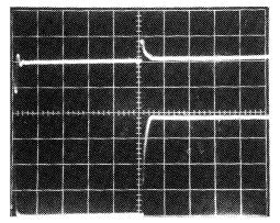
Top Trace: Output Voltage; 200mV/Div., 5μs/Div. Bottom Trace: Collector of load switching transistor, load = 1A; 5V/Div., 5μs/Div.
