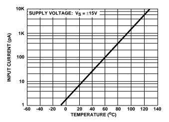
FIGURE 7. INPUT CURRENT vs TEMPERATURE
