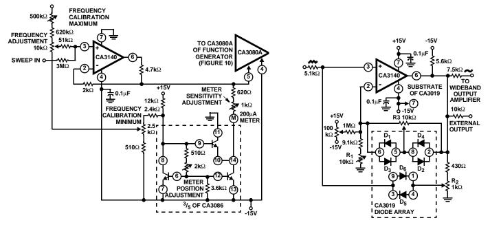
FIGURE 11. METER DRIVER AND BUFFER AMPLIFIER
