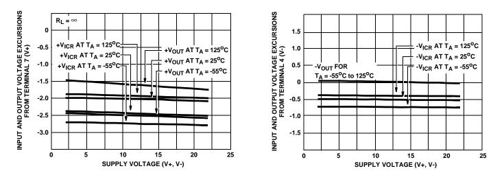
FIGURE 8. OUTPUT VOLTAGE SWING CAPABILITY AND COMMON MODE INPUT VOLTAGE RANGE vs SUPPLY VOLTAGE
